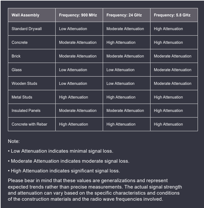
FIGURE 2: Visualization of the AI-generated chart detailing the various attenuation levels for signals on the 900mhz, 2.4Ghz, and 5.8Ghz radio frequencies.
